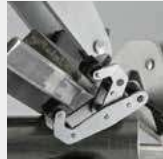
Smooth Surface For general purpose clamping.
